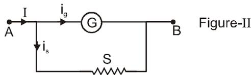
7. The resistance of the shunt 'S' and resistance 'G' of the galvanometer should have the following relation.
