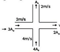
Sol. Inlet flow rate = Outlet flow rate  $(3A_0 \times 2) + (4A_0 \times 4) = (A_0 \times 2) + (2A_0 V)$   $22A_0 = 2A_0 + 2A_0 V$ V = 10 m/s
