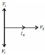
A) phase difference between current and voltage in a purely resistive AC circuit is zero.
