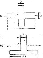
It is very clear that section modulus of section-II is more than that of section-III as more area is away from the neutral axis in section-II. Section-IV is unequal and its section modulus in tension and compression will be different. Since the strain is (I/E) at top most and at bottom most fibre it is less than I/E.
