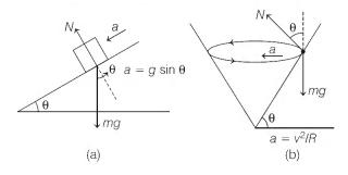
Net force perpendicular to acceleration should be zero. So, in the first figure,
