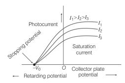
6. For a particular frequency of incident radiation, the minimum negative (retarding) potential  $V_0$  given to plate for which the photoelectric current becomes zero is called **cut-off** or **stopping potential**.
