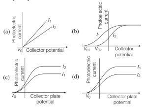
**49.** If collector plate is made negative with respect to emitter, at certain potential  $V_0$ , photocurrent is zero.
