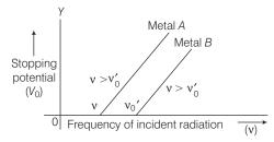
Variation of stopping potential  $V_0$  with frequency  $\nu$  of incident radiation for a given photosensitive material
