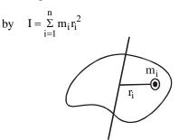
where  $m_i$  is the mass of  $i^{th}$  particle at a distance of  $r_i$ from axis of rotation.
