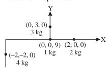
$$I = I_1 + I_2 + I_3 + I_4 = 0 + 0 + 27 + 16 = 43 \text{ kg m}^2$$
