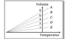
Solution : (d) From  $PV \propto MT$  or  $V \propto \frac{M}{P}T$ ; Here  $\left(\frac{M}{P}\right)$  represents the slope of curve drawn on volume and temperature axis.
