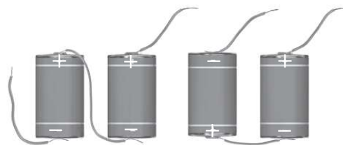
Connecting two cells together to make a battery
