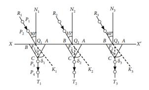
When viewed from the other face the pins are along a particular line. We place pins  $P_3$  and  $P_4$  in line with the images of  $P_1$  and  $P_2$  as seen in the prism. Thereafter line  $P_3P_4$  is drawn which represents the emergent ray.
