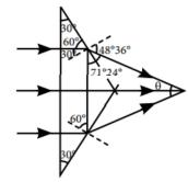
(b) : For total internal reflection at glass-air interface **64**. critical angle C must be less than 45°.
