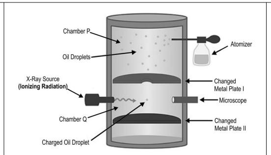
If it is observed that an ionized oil droplet having a mass of  $3.2 \times 10$ -14 kg and carrying a charge of -  $6.4 \times 10$ -19 C, remains stationary between the metal plates I and II when a potential difference 'V' is applied between the plates, then
