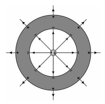
As the electric field outside the hollow conductor is not zero, it fails to shield its OUTSIDE from the electric field produced by the point charge on the inside.
