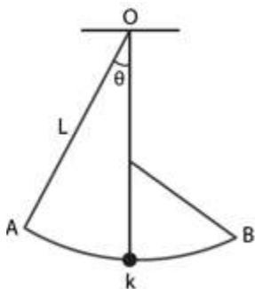
(a) When the height of the bob is less than the peg than the total potential energy of the bob at point A is equal to the potential energy of the bob at point B.
