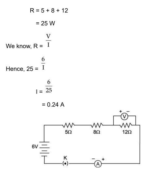
Since, resistances are connected in series, thus electric current remains the same through all resistors.
