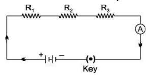
**Ans.** Let three resistors R1, R2 and R3 are connected in series which are also connected with a battery, an ammeter and a key as shown in figure. When key is closed, the current starts flowing through the circuit. Take the reading of ammeter. Now change the position of ammeter to anywhere in between the resistors and take its reading. We will observe that in both the cases reading of ammeter will be same showing same current flows through every part of the circuit above.
