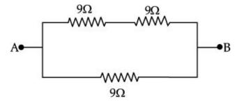
$R_{S} = R_{1} + R_{2}$ = 9 + 9 = 18 W
