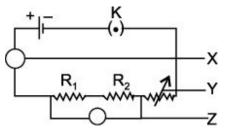
**Ans.** X = Ammeter, Y = Rheostat, Z = Voltmeter.
