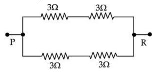
Equivalent resistance of two 3  $\Omega$  resistors connected in series is  $(3 + 3) = 6 \Omega$
