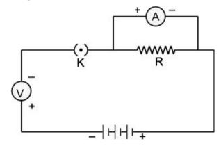
**Ans.** An electrical circuit is a continuous path comprising conducting wires and other electrical components between the terminals of a battery along which an electric current is set up. It is represented by drawing a circuit diagram.
