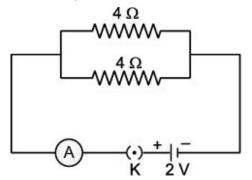
**Ans.** (a) The two resistors of resistance 4 W each are connected in parallel.
