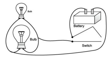
The reason for connecting the two bulbs in parallel is that (i) both the bulbs glow at the same voltage, and (ii) if one bulb stops glowing, the other bulb remains unaffected.
