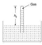
capacity of mercury, tube and the container are negligible. How much heat must be supplied to the gas inside the tube so as to increase its temperature by  $\Delta T$ ?
