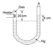
Area of cross section of the tube is uniform and is equal to 0.01 m<sup>2</sup>. The gas in the tube is heated by an electric heater so as to raise its temperature to 562.5 K. Assume that no heat is conducted to mercury by the gas.
