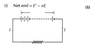
(ii) (a) Net internal resistance of the combination of cells = nrNet resistance = nr + R
