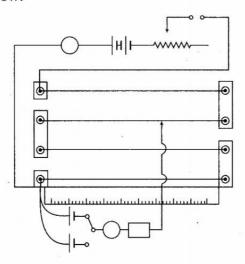
The main circuit comprises of battery of emf E, key (K) and rheostat  $(R_h)$ . The auxiliary circuit comprises of two primary cells of emfs  $E_1$  and  $E_2$ , galvanometer, jockey and resistance box (RB) to prevent large current flowing through the galvanometer.
