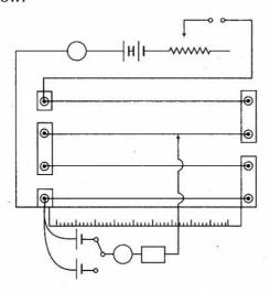
The main circuit comprises of battery of emf E, key (K) and rheostat  $(R_h)$ . The auxiliary circuit comprises of two primary cells of emfs  $E_1$  and  $E_2$ , galvanometer, jockey and resistance box (RB) to prevent large current flowing through the galvanometer.
