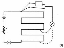
The cell of emf, E (internal resistance r) is connected across a resistance box (R) through key  $K_2$ .
