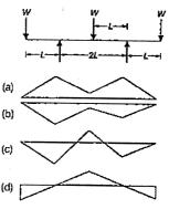
Q.19 Match List-I (Simply supported beams) with List-II (Shear force diagrams) and select the correct answer by using codes given below the lists:
