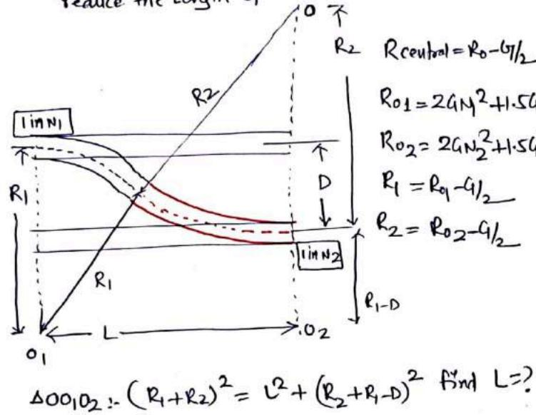
$$\Delta O_1 O_2 : (R_1 + R_2)^2 = L^2 + (R_2 + R_1 - D)^2 \text{ find } L=?$$
