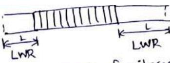
In case of LWR, the min. length of rail required to be welded at the end of track, so the portion of rail b/w welded rail does not undergo any thermal expansion/contraction is known as breathing Length.
