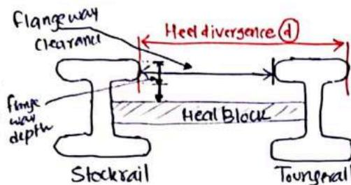
2- Flange way clearance :- distance b/w adjacent face of check rail and stock rail at heel of switch.
