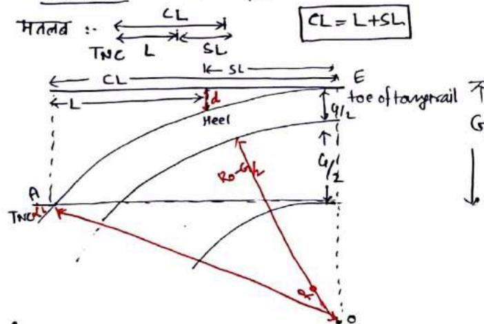
$$\left. \begin{array}{l} \text{outer radius } OA = OE = R_o \\ \text{central radius } R = R_o - G/2 \\ \text{heel divergence } 'd' = 13.3 - 13.7 \text{ BG (cm)} \\ \text{switch angle } \beta \text{ crossing angle } \alpha \end{array} \right\}$$
