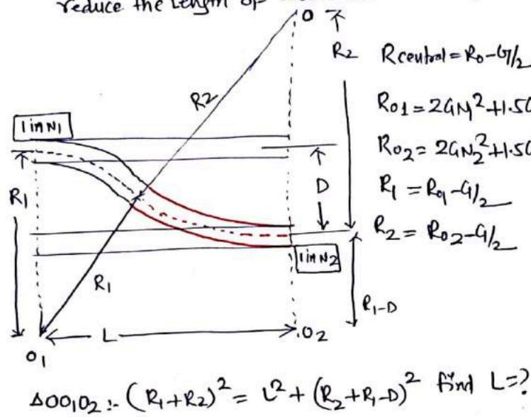
$$\Delta O_1 O_2 : (R_1 + R_2)^2 = L^2 + (R_2 - R_1/2)^2 \text{ find } L=?$$
