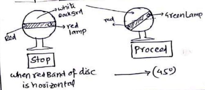
⑤ Calling on signals : use when repair work on
