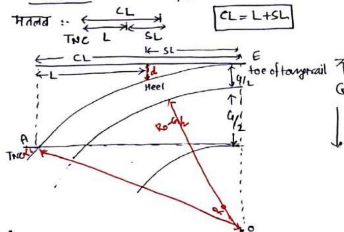
$$\left. \begin{array}{l} \text{outer radius } OA = OE = R_o \\ \text{central radius } R = R_o - G_1/2 \\ \text{heel divergence } 'd' = 13.3 - 13.7 \text{ BG (cm)} \\ \text{switch angle } \beta \text{ crossing angle } \alpha \end{array} \right\}$$
