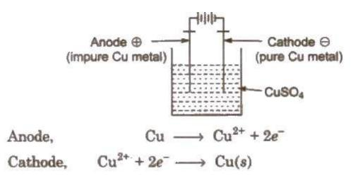
On passing electricity, the pure metal gets deposited on the cathode while the insoluble impurities settle down below the anode as anode mud or anode sludge. Metals like Cu, Ag, Au, Cr, Zn, Ni, etc are purified by this method.
