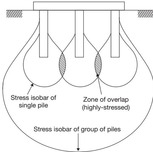
**Closely spaced group of piles (with zones of stress overlap)**
