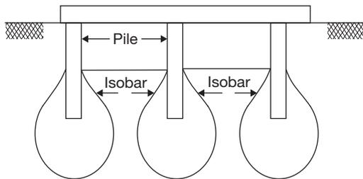
**Widely spaced group of piles (without zones of stress overlap)**
