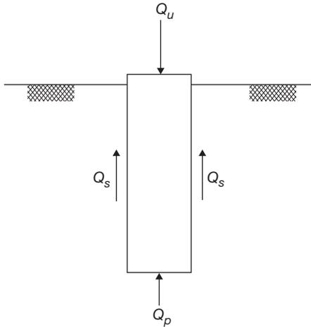
**Determination of  $Q_p$ :** The ultimate bearing capacity ( $q_p$ ) of the soil at the pile tip is similar to that of bearing capacity equation for a shallow foundation.
