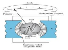
If k is torsional rigidity of material of suspension wire, then for deflection  $\theta$ , torque  $\tau$ . For equilibrium NIAB = k
