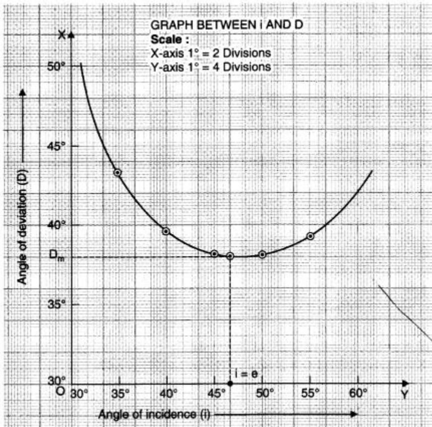
Fig. Graph between angle of incidence and angle of deviation.
