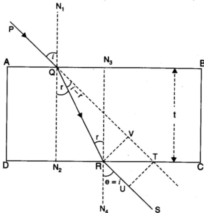
**Fig. 9.05.** Refraction through a glass slab.
