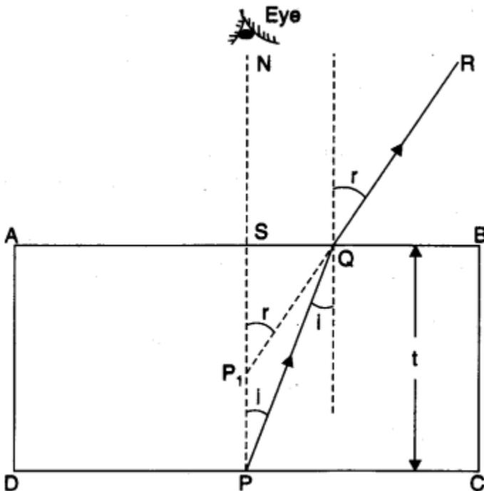
Fig. 9.06. Real and apparent thickness of a glass slab.
