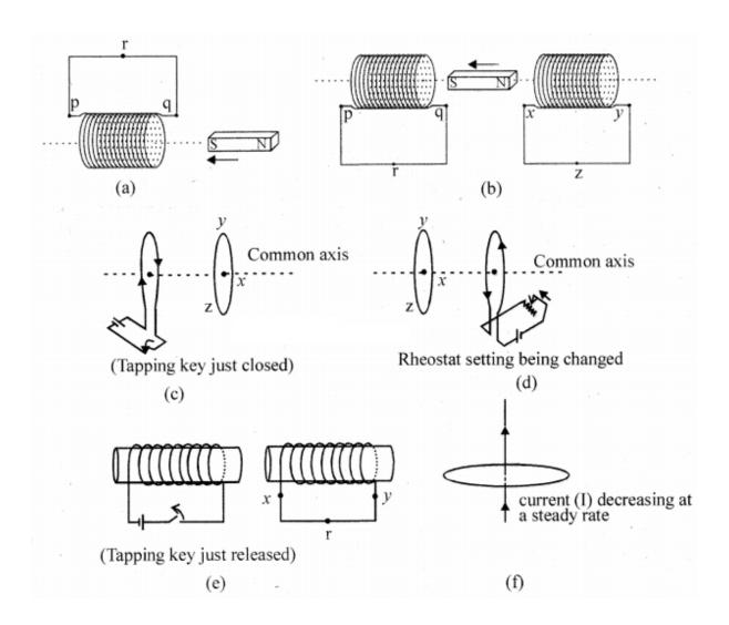
**Solution:** (a) According to Lenz's law, the end of the coil facing the S-pole of the magnet coil becomes an S-pole so as to repel the approaching magnet. For this to happen, the current in the coil will flow in the direction QRPQ.
