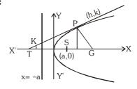
parabola are the bisectors of the angle between the focal radius SP & the perpendicular from P on the directrix. From this we conclude that all rays emanating from S will become parallel to the axis of the parabola after reflection.
