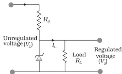
The unregulated dc voltage (filtered output of a rectifier) is connected to the Zener diode through a series resistance  $R_s$  such that the Zener diode is reverse biased.
