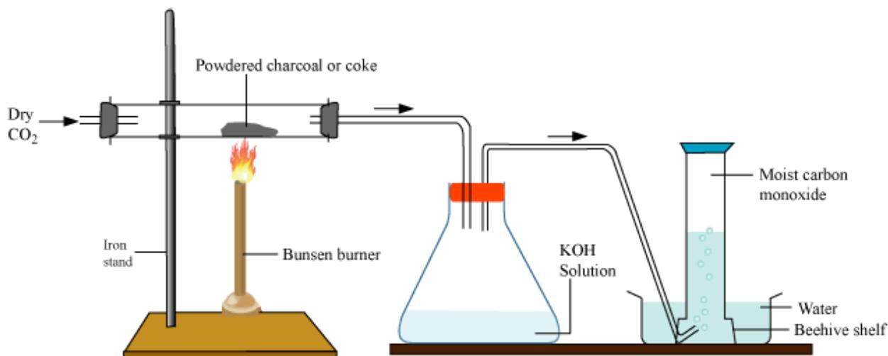
The charcoal is heated to a dull red heat and then carbon dioxide is passed over it.
