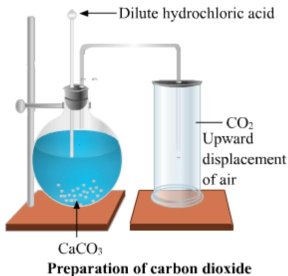
Take calcium carbonate ( $\text{CaCO}_3$ ) in the flask and start adding dilute HCl through the thistle funnel. When the reaction between  $\text{CaCO}_3$  and HCl takes place,  $\text{CO}_2$  is produced which is collected in the jar by upward displacement of air. The reaction involved is shown below:
