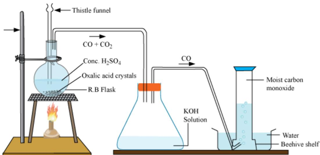
Pour concentrated sulphuric acid from thistle funnel so that the lower end of thistle funnel is completely immersed in acid. Heat the mixture.
