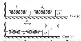
In case (ii), the springs are shown in the maximum compressed position. If the spring of spring constant  $k_1$  is compressed by  $x_1$  and that of spring constant  $k_2$ is compressed by  $x_2$  then
