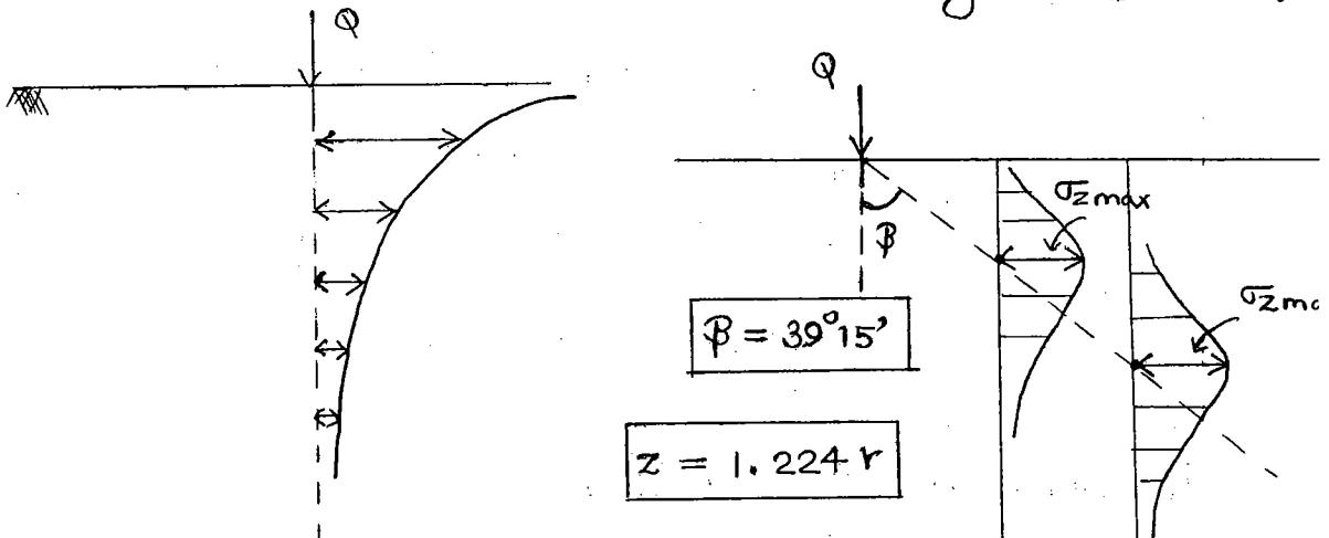
Q If a vertical plane is drawn at a radial distance of 2 m away from a vertical load at what depth max  $\sigma_z$  occurs.
