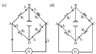
87. In the figure in balanced condition of wheatstone bridge
