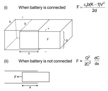
\* Force on the dielectric will be zero when the dielectric is fully inside.
