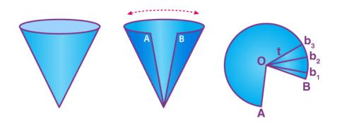
Label A and B and corresponding  $b_i$ ,  $b_a$  ... $b_n$  at equal intervals, with O as the common vertex. The Curved surface area(CSA) of the cone will be the sum of the areas of the small triangles:  $I/2 \times (b_i + b_a$ ...... $b_n) \times I$  (bl + b2...bn) is also equal to the circumference of base =  $2\pi r$  (On substituting the values)
