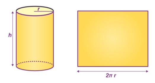
Curved surface area(CSA) of a cylinder of base radius r and height  $h = 2\pi \times r \times h$
