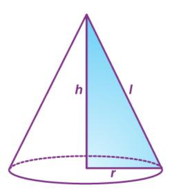
The relationship between slant height( $\hbar$ ) and height( $\hbar$ ) of a right circular cone is: a = ha + ra (Using Pythagoras Theorem)
