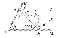
XA is the incident ray. BC is the final reflected ray. It is given that BC is parallel to mirror  $M_1$ . Look at the assignment of the angles carefully. Now  $N_2$  is normal to mirror  $M_2$ . Therefore  $\beta = \theta$
