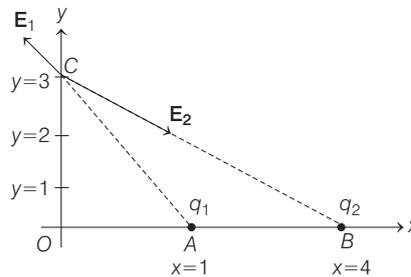
Let  $E_1$  and  $E_2$  are the values of electric field due to  $q_1$  and  $q_2$  respectively.
