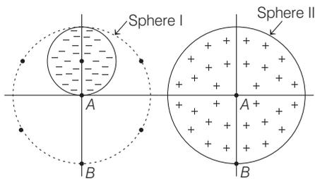
Now, electric field due to sphere I at points A and B are
