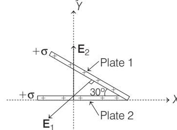
From geometry of figure, net electric field in region between plates is resultant of fields of both plates,
