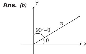
Torque applied on a dipole  $\tau = pE \sin \theta$  where,  $\theta =$  angle between axis of dipole and electric field.
