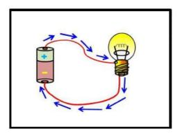
**Fused:** An electric bulb is said to be fused when it is connected to a cell in a circuit but does not glow. An electric bulb may fuse due to many reasons like if the filament of the bulb is broken the bulb does not glow.
