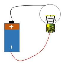
**Solution:** No. The bulb does not glow in this case. For a bulb to glow, the positive terminal of a battery is to be connected with one terminal of the bulb and the negative terminal of the battery is connected with other terminal of the bulb.
