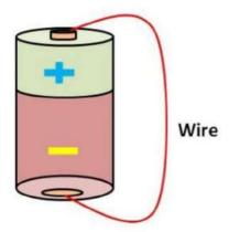
**Solution:** When we join the two terminals of the electric cell without connecting them through a switch and a device like a bulb, then the maximum possible current flows through the circuit. Because of this, the chemical energy stored in the cell gets used up very fast which gets converted to electricity. This results in the capacity of the cell getting quickly diminished.
