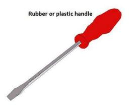
**Solution:** Rubber and plastic are bad conductors of electricity. It does not allow current to flow through it. Hence, handles of tools such as screwdrivers which are used by electricians usually have plastic or rubber cover on them. This protects them from any electric shock.
