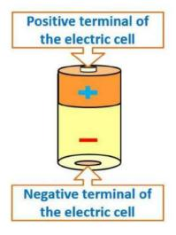
**Tip:** Never join the terminals of the electric cell because in this case electric cell get used up very fast and the cell stop working.
