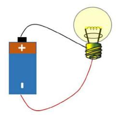
**Electric Circuit:** When electric components like bulb, cell, wires etc. are connected with each other, the setup is called an electric circuit.
