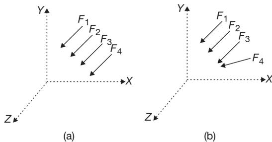
**6. Like parallel and unlike parallel force systems:** In a like parallel force system (Figure (a)), the lines of action of the entire constituting forces are parallel to each other and act in the same direction. In an unlike parallel force system (figure), the lines of action of the entire constituting forces are parallel to each other, where some of them act in different directions.
