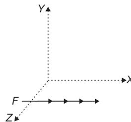
4. **Concurrent and non-concurrent force systems:** If the lines of action of all the forces in a force system pass through a single point, then the force system is called a concurrent force system (Figure (a)), else it is called a non-concurrent force system (Figure (b)).
