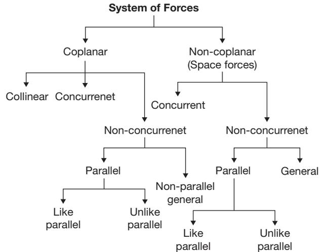
2. **Coplanar and non-coplanar (spatial) force systems:** In a coplanar force system (Figure (a)), the constituting forces have their lines of action lying in the same plane. If all the lines of action do not lie in the same plane, then the corresponding forces constitute a non-coplanar force system (Figure (b)).
