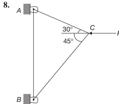
Two steel truss members AC and BC with cross section area  $100 \text{ mm}^2$  is subjected to a horizontal force P kN as shown in figure. Maximum value of P such that axial stress in any of the members does not exceed 50 MPa is
