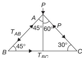
$$T_{AB} \cos 45^\circ + T_{AC} \cos 60^\circ - P = 0$$
