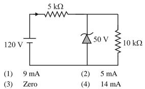
**9.** In the given circuit the current through Zener Diode is close to:
