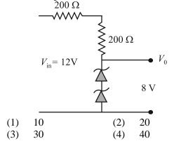
4. The reverse breakdown voltage of a Zener diode is 5.6 V in the given circuit.
