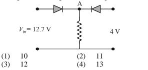
**3.** The circuit shown below is working as a 8 V dc regulated voltage source. When 12 V is used a input, the power dissipated (in mW) in each diode is; (considering both zener diodes are identical) \_\_\_\_\_.
