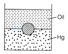
$$\Rightarrow V\rho g = \rho_{\text{oil}} \times \frac{V}{2} \times g + \rho_{\text{Hg}} \times \frac{V}{2} \times g$$
