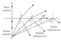
Critical angle: It is that angle of incidence for which the angle of refraction
