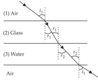
$$^{1}\mu_{2} = \frac{\sin i_{1}}{\sin r_{1}}, ^{2}\mu_{3} = \frac{\sin r_{1}}{\sin r_{2}} \text{ and } ^{3}\mu_{1} = \frac{\sin r_{2}}{\sin i_{1}}$$
