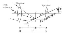
Construction for compound microscope:
