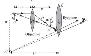
Angular magnification,  $m = \frac{v_0}{u_0} \left( 1 + \frac{D}{fe} \right)$
