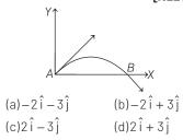
Concept As we know that in projectile motion only velocity of y component change, whereas velocity of x component remains constant. From the figure, the x-component remains unchanged, while the y-component is reversed. Thus, the velocity at point B is  $(2\mathbf{i} - 3\mathbf{j})$  ms<sup>-1</sup>.
