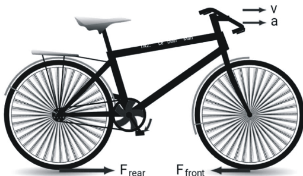
Friction Force on the Wheels during Pedaling
