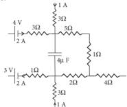
Calculate the energy stored in the capacitor  $C(4 \mu F)$ .
