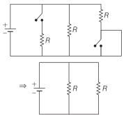
So, equivalent resistor  $=\frac{R}{2}=\frac{9}{2}$  ohms
