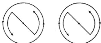
Hence, current loop have both magnetic poles and therefore, behaves like a magnetic dipole
