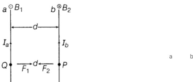
Let  $a$  and  $b$  be two long straight parallel conductors.  $I_a$  and  $I_b$  are the current flowing through them and separated by a distance  $d$ . Magnetic field induction at a point  $P$  on a conductor  $b$  due to current  $I_a$  passing through  $a$  is
