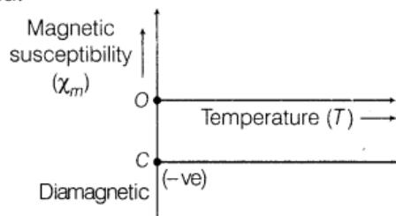
This is the graph for variation of  $\chi_m$  with temperature ( $T$ ) of diamagnetic substance for material  $B$ . (1)
