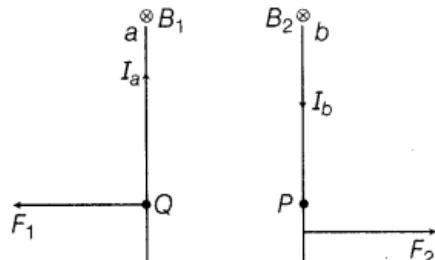
Now, let the direction of current in conductor  $b$  be reversed. The magnetic field  $B_2$  at point  $P$  due to current  $I_a$  flowing through  $a$  will be downwards. Similarly, the magnetic field  $B_1$  at point  $Q$  due to current  $I_b$  passing through  $b$  will also be downward as shown. The force on  $a$  will be, therefore towards the left. Also, the force on  $b$  will be towards the right. Hence, the two conductors will repel each other as shown.
