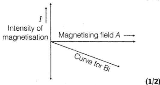
The diamagnetic material exhibits perfect conductivity (superconductivity) and perfect diamagnetism when metal is cooled below the critical temperature of the material (Meissner effect). (1)
