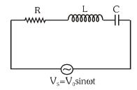
Impedance of circuit  $Z = \sqrt{R^2 + X^2} = \sqrt{R^2 + \left(\omega L - \frac{1}{\omega C}\right)^2}$
