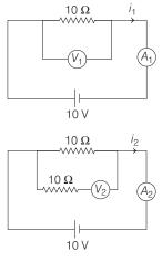
(a)  $V_1 = V_2$  and  $i_1 > i_2$  (b)  $V_1 = V_2$  and  $i_1 = i_2$ (c)  $V_2 > V_1$  and  $i_1 > i_2$  (d)  $V_2 > V_1$  and  $i_1 = i_2$
