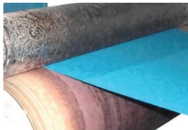
Figure 1.4 Fabric Embossing Machine
