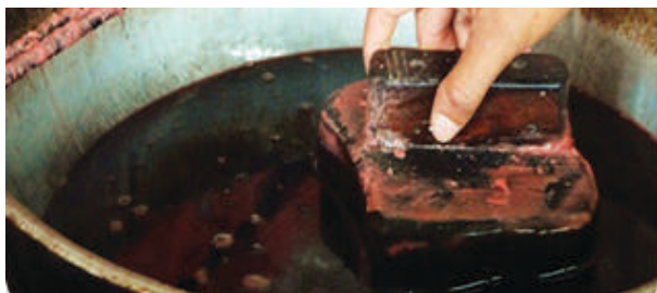
Figure 3.17 Nail Block in Wax for Batik Printing
