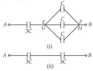
The equivalent capacitance between A and B is  $\frac{1}{C_{\text{eq}}} = \frac{1}{3C} + \frac{1}{3C}, \frac{1}{C_{\text{eq}}} = \frac{2}{3C}, C_{\text{eq}} = \frac{3}{2}C = 1.5C$
